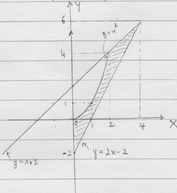
① Revolution about  $X$ -axis (cylindrical shell method)
