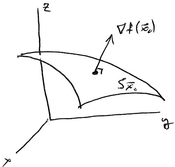
Another way to say this is that, any vector  $\vec{v}$  tangent to  $S_{\vec{x}_0}$  will be perpendicular to  $\nabla f(\vec{x}_0)$ .
